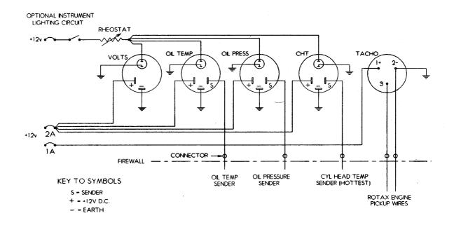
Fig 2. Rotax 912 instrument wiring diagram.
