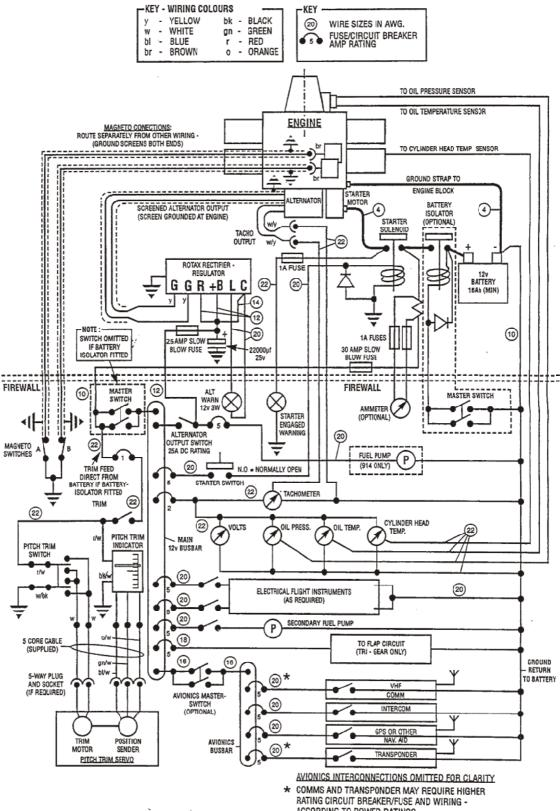
IMPORTANT : ENGINE RELATED WIRING MUST COMPLY WITH ROTAX INSTALLATION MANUAL
